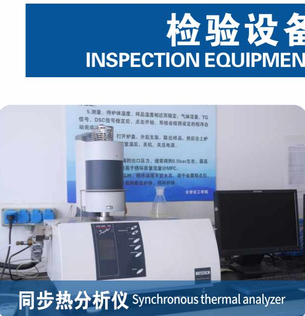
**同步热分析仪** Synchronous thermal analyzer
