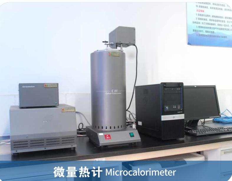
**微量热计** Microcalorimeter
